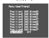
3 Use the [ ▲ ] [ ▼ ] buttons to turn the switching function on/off.
